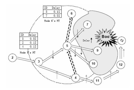
Figure 3 Backpressure Re-Routing [35]
