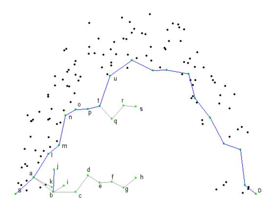
Figure 18 Message Transmission using PGR
