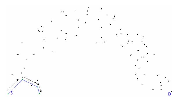
Figure 11 Example of Topology leading to failure of BGR
