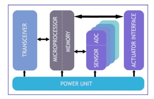
Figure 2 Structure of a Sensor Node
